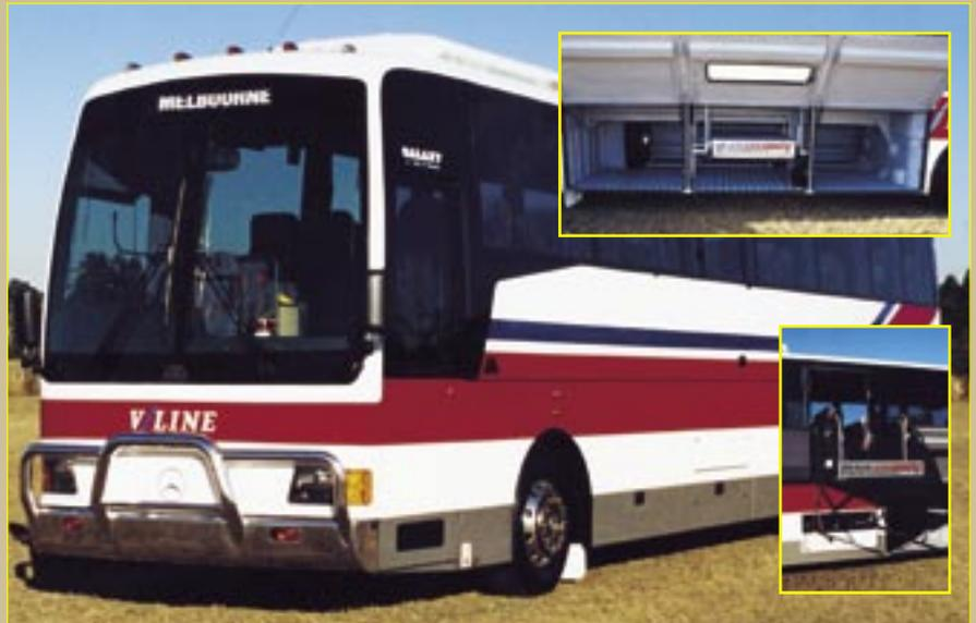
**Cost effective dignified means of loading and unloading disabled people. The cassette can be removed to maximise bin space and minimize weight and can be interchanged between similar set up vehicle therefore reducing capital costs**
